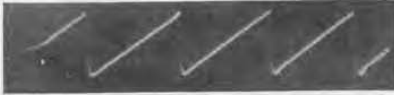
FIGURE 5. Output waveform of one TYPE 506-A Sweep Circuit as shown on the cathode-ray oscillograph using another to supply the linear time axis. Note the close approach of each trace to the ideal straight line
