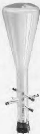
FIGURE 1. The General Radio cathode-ray oscillograph tube. The inside of the glass at the large end is coated with a fluorescent substance on which the moving beam of electrons traces patterns
