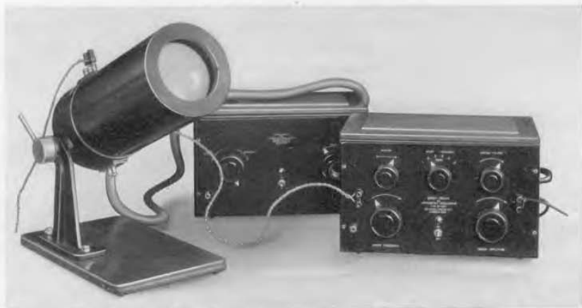
FIGURE 7. The TYPE 506-A Sweep Circuit is shown at the right of the mounted oscillograph tube and its a-c operated power supply equipment
